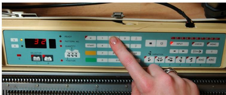
The number of available rows in the machine's memory will appear on the display. Press CE to clear the display.
