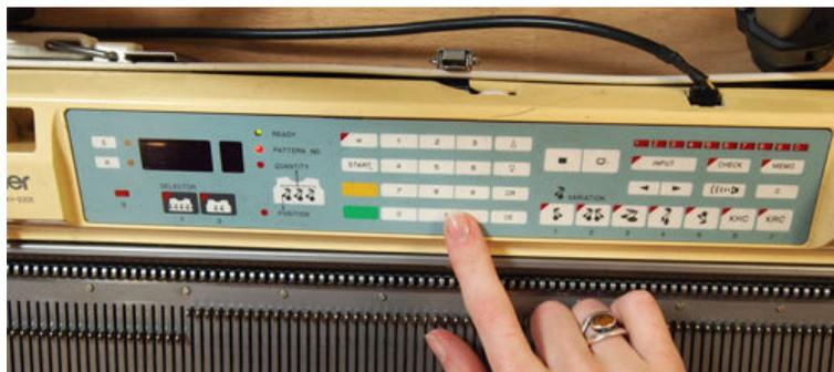
Press 1 to indicate which "track" to load from the disk drive emulator, then press STEP.
