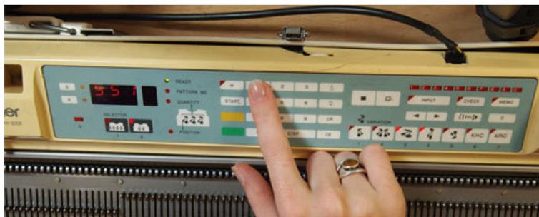
Display should go blank, then "ready" and "pattern no" lamps should illuminate.
